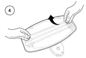
**4.** Carefully remove the bulbs and replace with the correct quartz bulbs.
