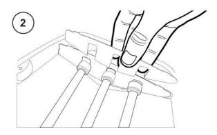
2. Remove the metal plate surrounding the end of the bulbs as shown. The use of a flathead screwdriver may be needed to open up the small metal tab on the top. Repeat for the other end.
