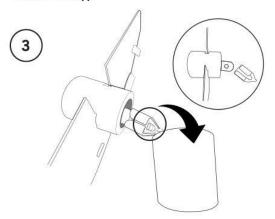
**3.** Slide the rubber caps off the bulb connectors and press the small tab (circled) to disconnect from the bulbs. Repeat for the other end.
